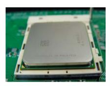
5. Gently press the CPU socket lever down until it locks in the plastic tab.
